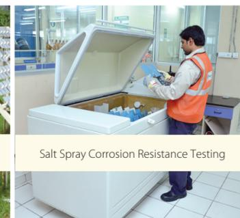
Salt Spray Corrosion Resistance Testing
