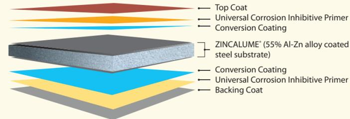
Cross Section View of COLORBOND® steel
